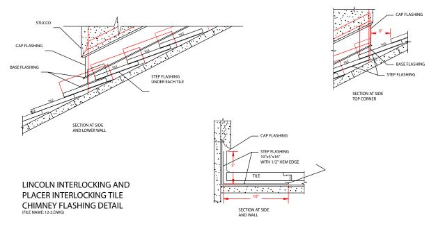
Base flashings, step flashings, and cap flashings around chimney walls should follow procedures illustrated in these drawings.
